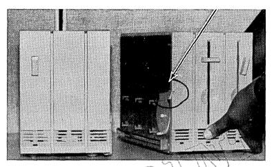
Push the modules together. It may help to mate the back of the two modules first and then move them together at the front.
