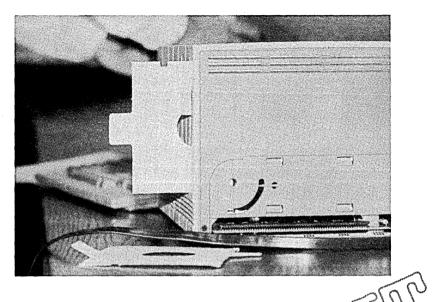
Remember to reinsert the shipping cards while the Floppy Disk Drive Module is moved to another location.
