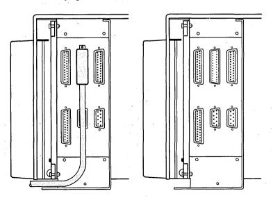
Remove the Monochrome Monitor cable from the Processor Module I/O panel and plug it into the connector on the I/O panel of the Graphics Controller Module. Use a small screwdriver to tighten the screws at the top and bottom of the plug.
