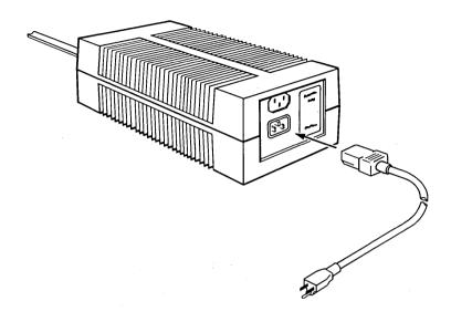
Plug the flat power cable from each additional 36-Volt Power Supply into any module that causes the cumulative 36-Volt Power Supply power code to exceed 10. Plug the female end of an additional ac line cord into the ac jack on the 36-Volt Power Supply.
