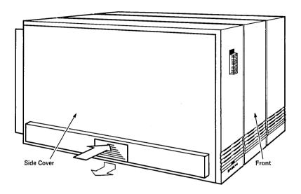
Pull the side cover down and off to reveal the three Memory Expansion Cartridge slots.
