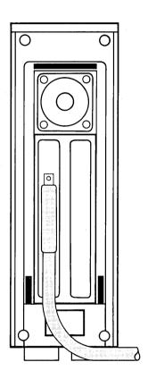
Replace the I/O cap on the rear panel by sliding the top of the cap up and into the slot near the top of the rear cover. rotate the cap downward to the vertical position and snap the hooks near the bottom of the I/O cap into place in the rear cover.
