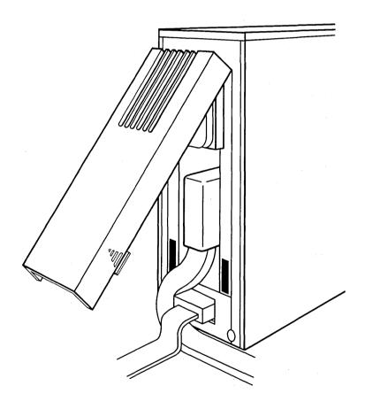
When the cable is routed correctly, it will be easier to replace the I/O cap on the rear panel. Replace the I/O cap on the rear panel by sliding the top of the cap up and into the slot near the top of the rear cover. Then rotate the cap downward to the vertical position and snap the hooks near the bottom of the I/O cap into place in the rear cover.
