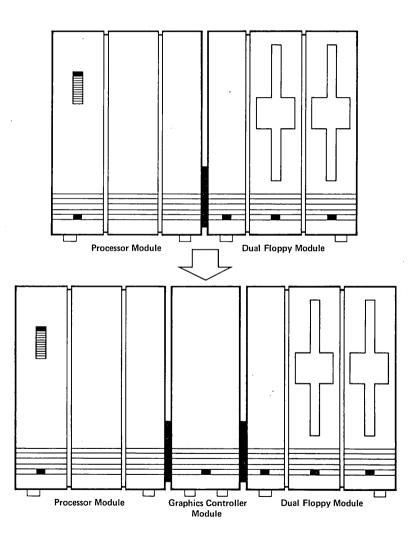
Connect the Graphics Controller Module to the workstation as described in Section 3, "Module Connection."
