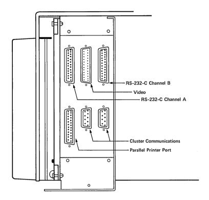
As the cables are plugged into their connectors, feed the cables through the cable exit runway provided underneath the back of the Processor Module.
