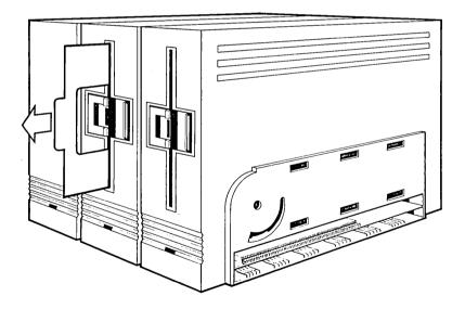
Remove the two cards (one in each drive). These cards protect the read/write heads in the floppy disk drives during shipment. The read/write heads will be damaged if the cards are not removed before you power up the workstation.
