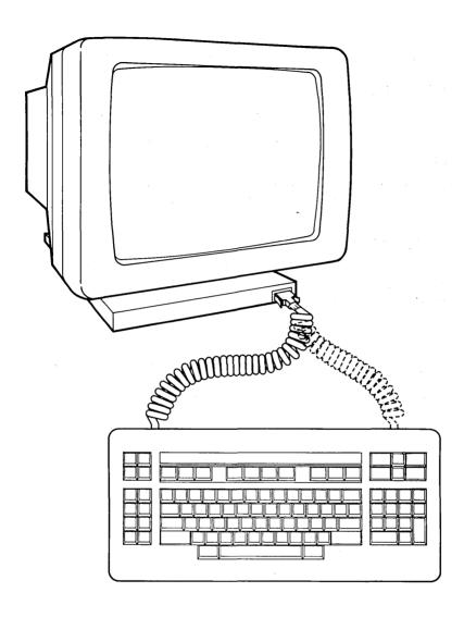
Next, push the other end of the keyboard cable into the monitor jack at the front edge of the monitor. The connector fits into the monitor jack only one way. You should hear a click when the connector is inserted correctly.
