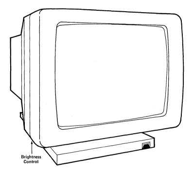
To adjust the viewing angle of the monitor, grasp both sides of the monitor housing and tilt it for the most comfortable viewing position.
