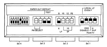
Dark indicates down. Switches where setting is not indicated depend on print thimble. See NEC documentation.
