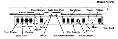
Figure D-1. Sprint 5 Printer Switches.
