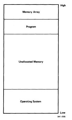
Figure 4-2. A Program with the Memory Array.
