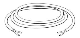
Insulation Removed from New Piece of Cable
