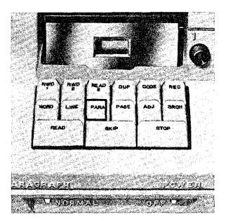
(1) With the Paragraph Control Key lighted, depress Read to read out the first paragraph. Where does the typesphere stop?
