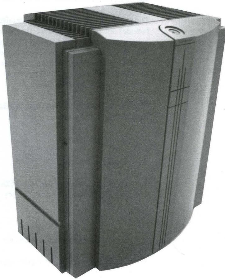
Figure 1-1. CRAY Y-MP EL Computer System
