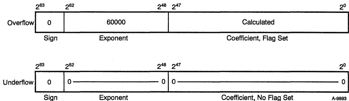
Figure 2-8. Floating-point Add and Multiply Range Errors
