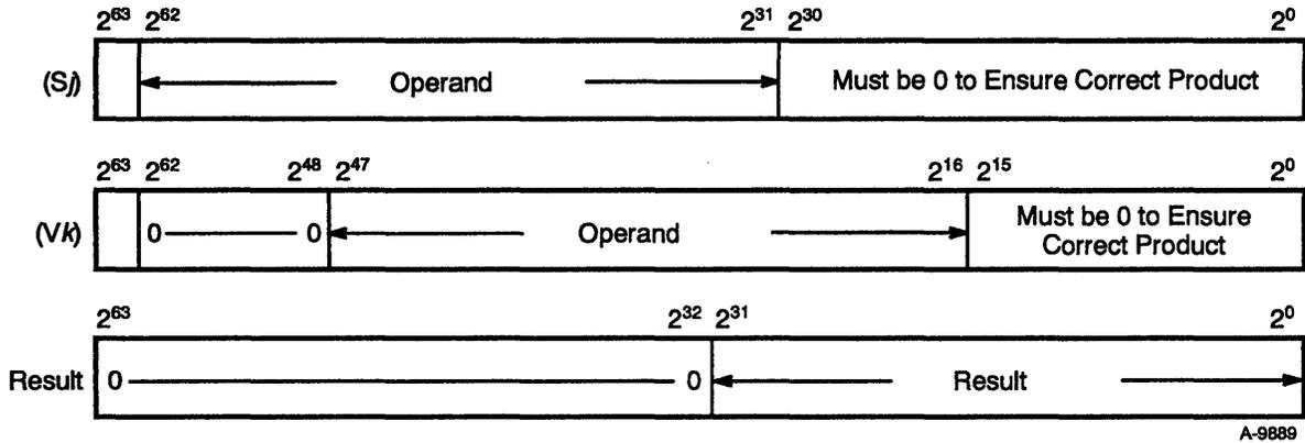
Figure 2-4. 32-bit Integer Multiply Performed in Floating-point Multiply Functional Unit
