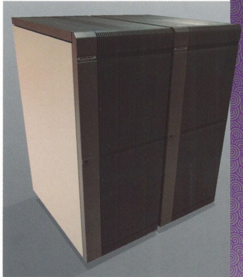
Two DE-60 disk cabinets, each containing up to eight DD-60 or DD-61 disk drives.
