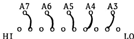
If other port addresses are desired, these traces must be cut and the other corresponding addresses jumped appropriately.
