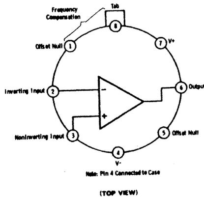
The leads of the TO-5 style ICs should be shaped into two rows of four and inserted into the IC socket in this order:
