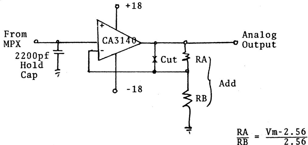
Changing the amplifiers to  $\pm 18V$  power requires cutting the power traces on the PCB and installing appropriate jumpers. Pads are provided for installation of the resistors RA and RB. A trace on the PCB solder side must be cut to permit RA to function.
