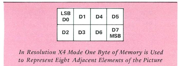
The 2K byte Dazzler picture is stored in memory as four quadrants. Each quadrant of the picture occupies one 512-byte page of memory. Only one page of memory is displayed for a 512-byte picture. The sequence in which memory is scanned in making a 2K byte picture is shown below:
