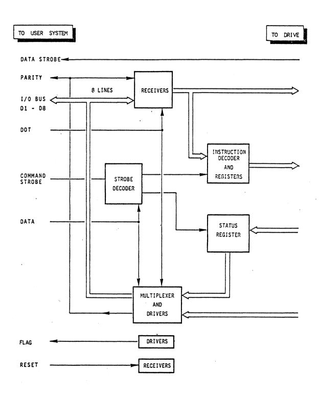
Figure 6. Real Time controller interface circuits
