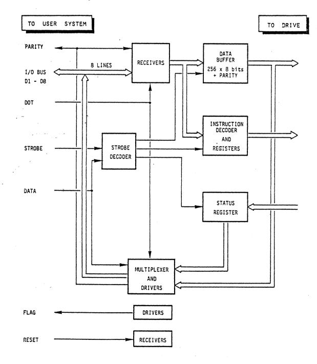
Figure 5. Buffered controller interface circuits
