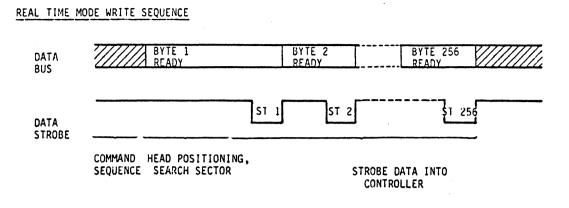
Figure 11. Write operation - real time mode
