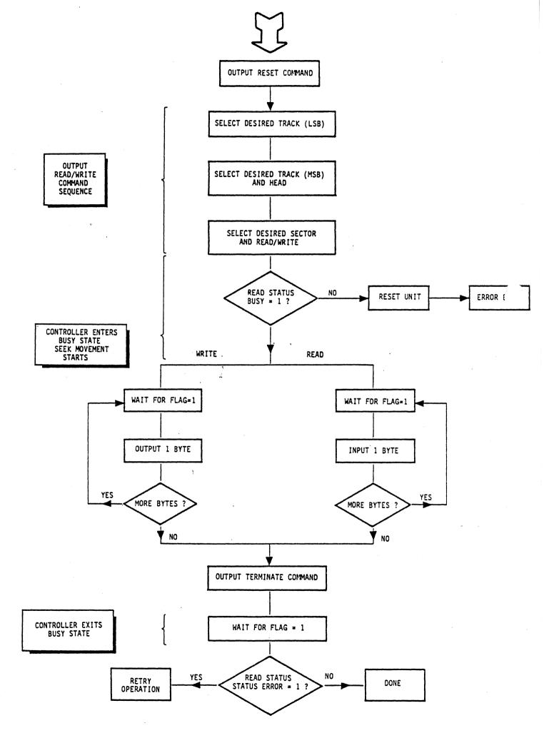
Figure 16. Read/write operation flowchart - buffered mode - 28 -
