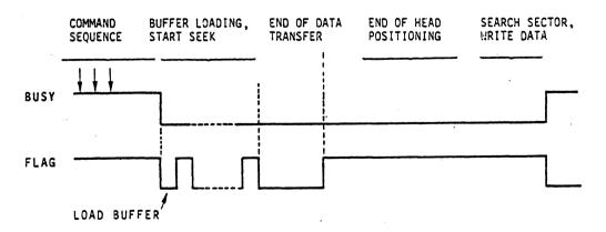
Figure 10. Write operation - Buffered mode
