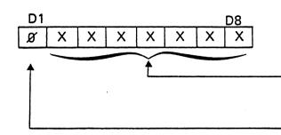
bits 2 to 8 may be 1 or 0, and signify the seven low order bits of the track address. bit D1 is always 0
