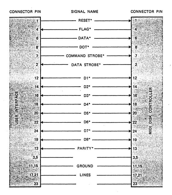
Figure 4. Interface signals and pin. Nos. - Real Time Mode
