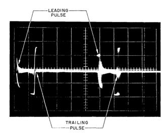
Figure 6-10 Proper Delay Adjustment Showing Equal Positive and Negative Trailing Pulse
