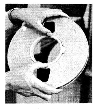
Figure 3-2 Installing the Write Enable Ring
