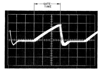
Figure 6-7 Read Control Delay Set to One Half Bit Period
