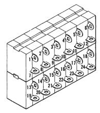
TRANSPORT MATING CONNECTOR - ELCO RF22420-5 CONNECTS TO P1 ON TRANSPORT CONTROL CABLE
