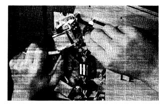
Figure 6-15 Loosening Pinchroller Shaft Screws
