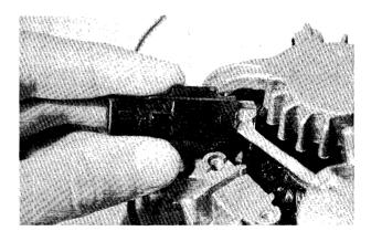
Figure 6-30 Removing Connecting Clip From Brushholder
