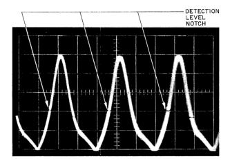
Figure 6-6 Signal Rectifier Output Showing Detection Level at 40%
