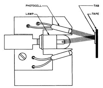
Figure 5-13 Photosense Head
