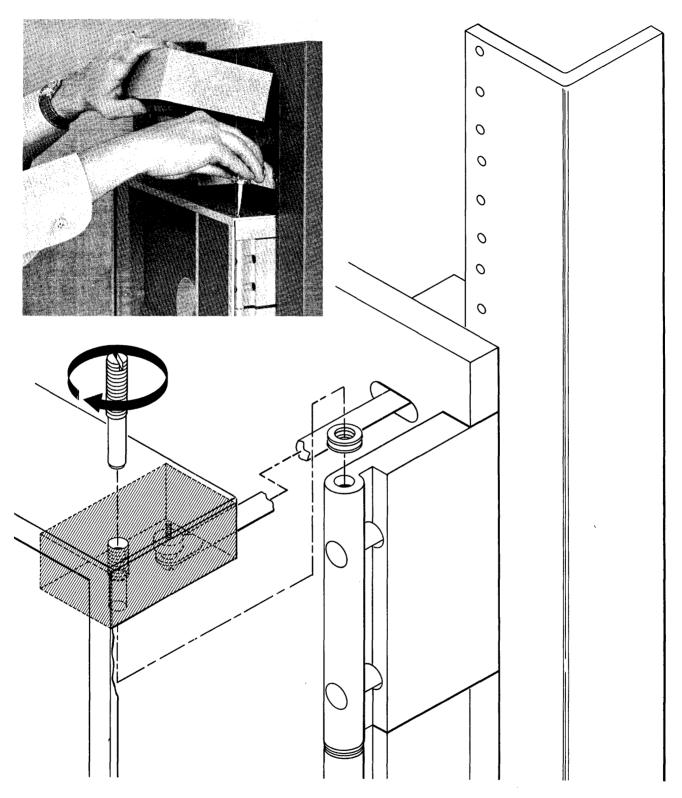
Figure 2-15 Cover Door Installation
