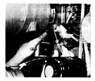
Figure 6-26 Adjusting the Running Vacuum
