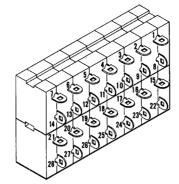
CONTROL CONNECTOR - ELCO RF22824 Connects to J2 on Operator Control Panel
