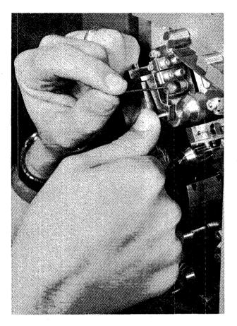
Figure 6-17 Applying Preload to Pinchroller Bearings
