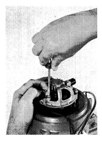
Figure 6-29 Removing Brush Holder Retaining Clip
