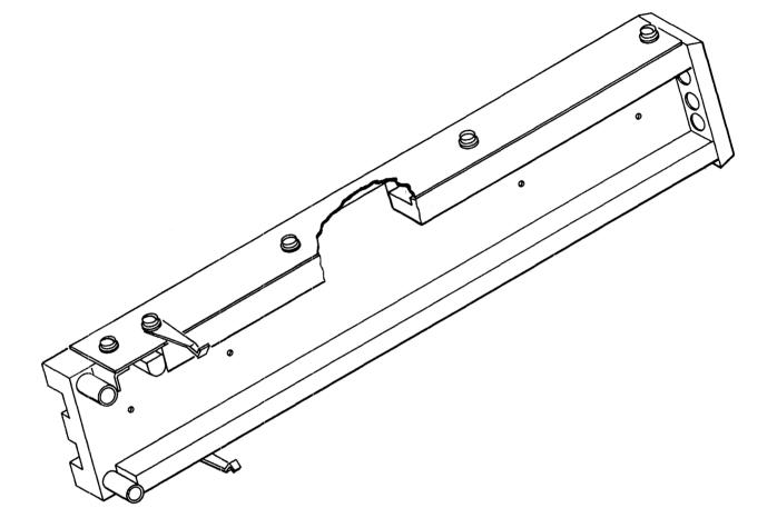
Figure 5-5 Vacuum Chamber (Take-up Reel)
