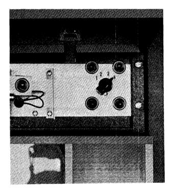
Figure 3-8 Tape Unit Address Designator Switch
