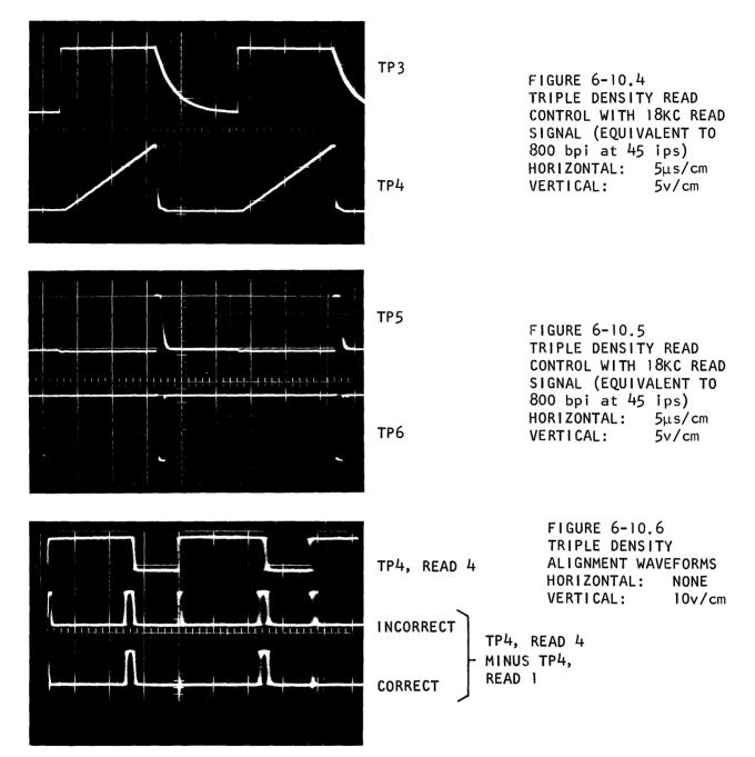
signals, as shown in Figures 6-10.1 through 6-10.3 for 800 bpi at 45 ips.
