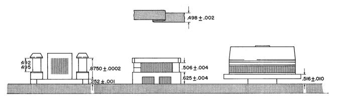
Figure 6-11 Critical Tape Path Dimensions
