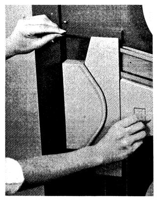
Figure 3-4 Pulling the Tape from File Reel
