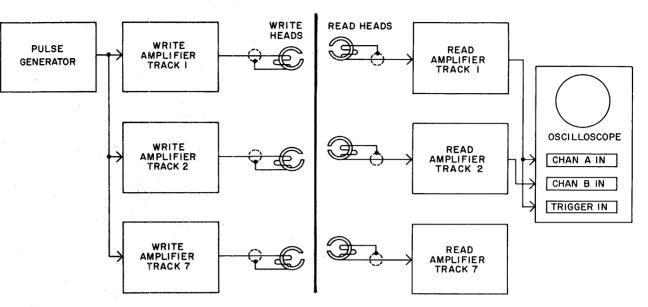
Figure 4-6 Test Set-Up for Checking ICTDE (Step 2)
