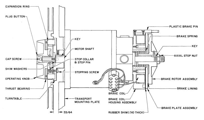
Figure 5-2 Supply Reel Motor Assembly
