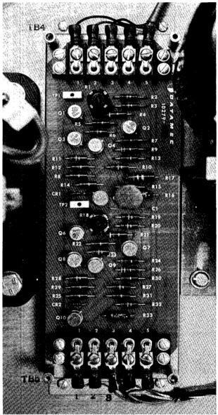
Figure 5-14 Photosense Amplifier
