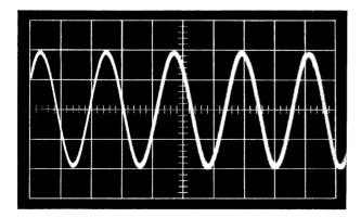
Figure 6-5 Preamp Output, Set to 8v. Peak to Peak
