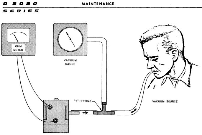
Figure 6-23 Testing Vacuum Switches
