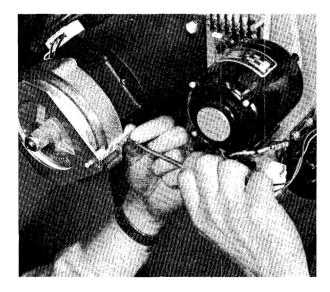
Figure 6-4 Adjusting the Drag Brake
