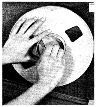
Figure 3-3 Installing the File Reel
