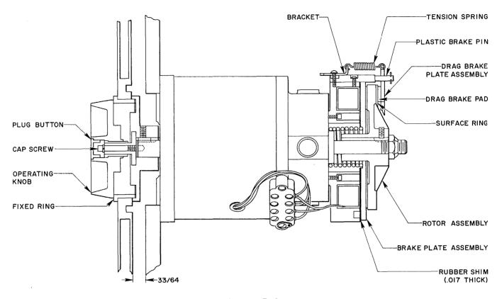
Figure 5-3 Take-up Reel Motor Assembly
