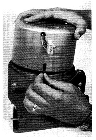
Figure 6-27 Removing Vacuum Unit Cover
