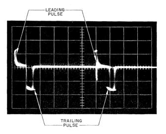
Figure 6-8 Delay Adjustment Showing Trailing Pulse Negative
