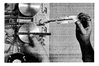
Figure 6-20 Measuring Capstan Belt Tension
