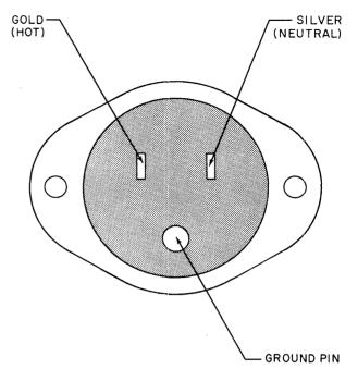
Figure 2-2 Power Line Connections
