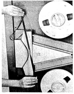
Figure 3-5 Threading the Tape (Step 6)
