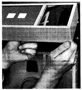
Figure 3-9 Removing or Installing Illuminated Number
