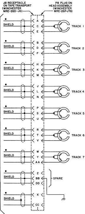
FIGURE 2-13 HEAD CONNECTOR WIRING (WRITE)
