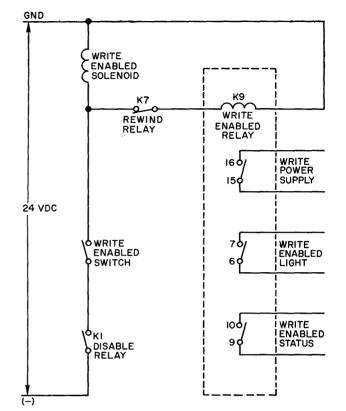
Figure 5-11 File Protect Schematic
