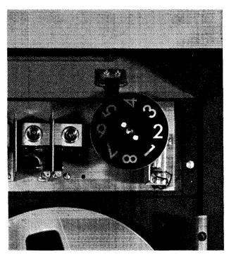
Figure 3-10 Operator Control Panel With Number Wheel
