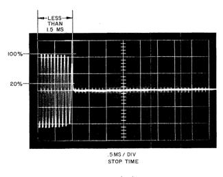
Figure 4-4 Stop Time reverse stop characteristic, which should resemble Fig. 4-4. Stop time, as determined from the oscilloscope display, should be less than 1.5 msec.
