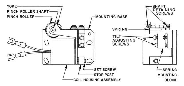
Figure 5-7 Actuator Assembly
