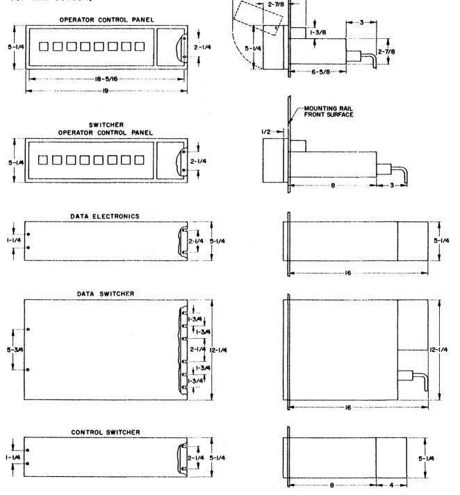
Figure 2-7 Mounting Dimensions (Sheet 2)
