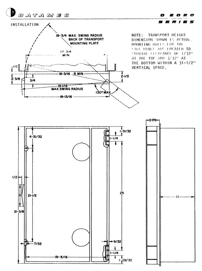
Figure 2-7 Mounting Dimensions (Sheet 1)
