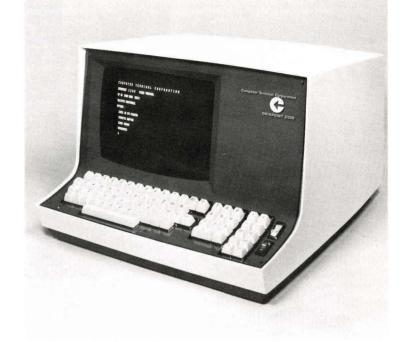
in a single glance and where necessary to make modifications and revisions. Program debugging is greatly simplified. With the 3300, the remote computer becomes a much more flexible aid to human thought processes. Data transmission rates of up to 2400 bits per second are available on the Datapoint 3300.
