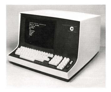
Many options are available for this terminal, one of which is Auto-Tab. This option extends the flexibility of the 3360 Terminal by providing direct cursor positioning to any location directed by program control. This option will also allow the terminal to search out and locate for program control the exact location of three separate and distinct symbols and multiple locations of these symbols.
