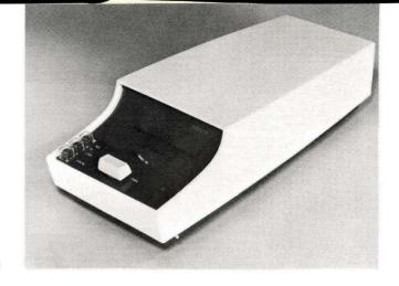
Reproduce-Remote Mode — The Tape Unit is placed under the control of the communications interface system of the CRT Terminal. Data is reproduced in start-stop format at the speed setting of the interface. The "X-on", "X-off" controls may be applied to provide automatic computer access of a message prepared off-line. The data is also displayed on the CRT during transmission.
