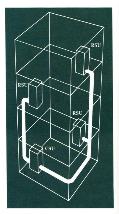
The dispersed architecture of the ISX lets you connect a Central Switching Unit with multiple Remote Switching Units placed where they can serve your business telephone and information switching needs most effectively.
