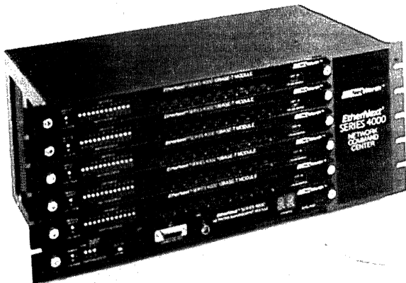
The EtherNext 4000 Network Command Center is a six-slot chassis. It is shown here with five UTPM12 10BASE-T modules and an NMM01 Network Management Module installed.
