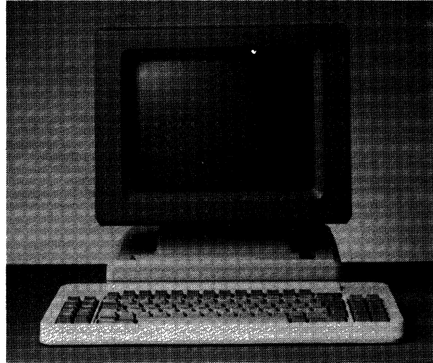
ITT Courier's 1700 Display Terminal is functionally compatible with the IBM 3178. The 1700 features a 12-inch tilt/swivel screen, and a detached low-profile keyboard. The terminal's footprint measures 13 inches by 12 inches, and the keyboard is 16 inches wide.
