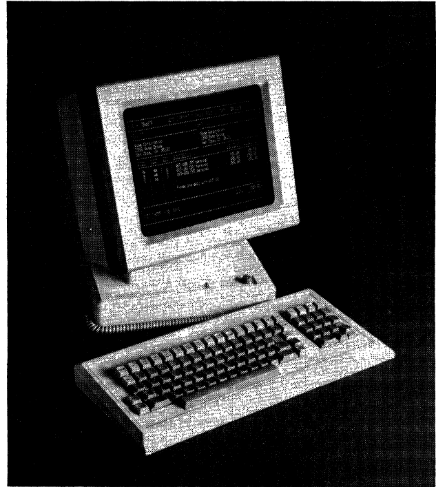
Qume's QVT 103 display provides emulation of the DEC VT100 and VT131. The QVT 103 features ANSI X3.64 command code compliance, selectable 80/132-column display capability, and ergonomic features such as a tilt/swivel display and a detachable keyboard. The QVT 103 can be selected with a 12-inch (standard) or 14-inch (optional) screen size.
