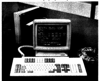
The Harris H191 Display Terminal is IBM 3191 compatible with a 12- or 14-inch monitor and a 1,920-character screen. The H191 offers screen printer support, light pen support, and extended highlighting.
