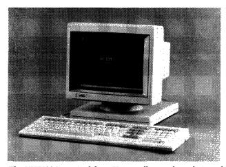
The UVT1224 terminal from Unisys offers total emulation of Unisys SVT1220 and is compatible with Digital Equipment's VT52, VT100, and VT220 video terminals.
