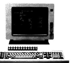
The IBM 3180 Display Station offers a 15-inch adjustable display unit, a logic element that snaps onto the back of the CRT, and a modifiable keyboard.
