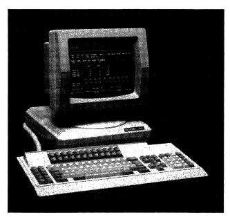
The Memorex 2291 Display Station has a 122-key modifiable keyboard, screen printer support, and modular design and is a plug-compatible replacement for the IBM 3191 Display Station.
