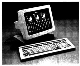
The Wyse WY-50 is a full-function, general-purpose ASCII terminal with 80-/132-column tilt/swivel display. Other features include multiple emulations and 16 dedicated function keys.
