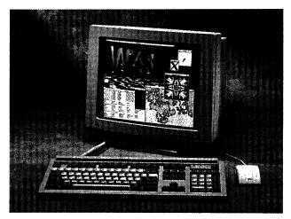
Wyse Technology's X terminal, the WY-X5, includes a flat, 17-inch, noninterlaced monochrome display with amber-white characters. The screen provides a 1,280-by-1,024 pixel resolution, 108 dots per inch, and a 70 Hz flicker-free refresh rate. Intuitive setup menus provide easy access to a variety of features, including configuration parameters, diagnostics, and network statistics.
