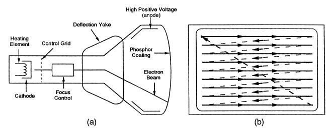
(a) The CRT produces images by generating a beam of electrons and focusing it onto a phosphorous-coated screen, which fluoresces or emits light at the point of contact. (b) The beam sweeps the screen from top to bottom and left to right in a pattern called a raster scan.
