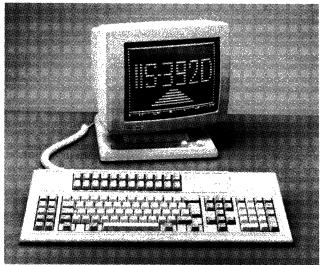
The Intelligent Information Systems (IIS) Model IS-392D is plug compatible and interchangeable with the IBM 3192 Model D Display Station. The terminal features four user-selectable screen formats and extended data highlighting facilities.
