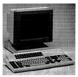
The IDEA 9291 Monochrome Display is an IBM coax-compatible display comparable to the IBM 3191 model.
