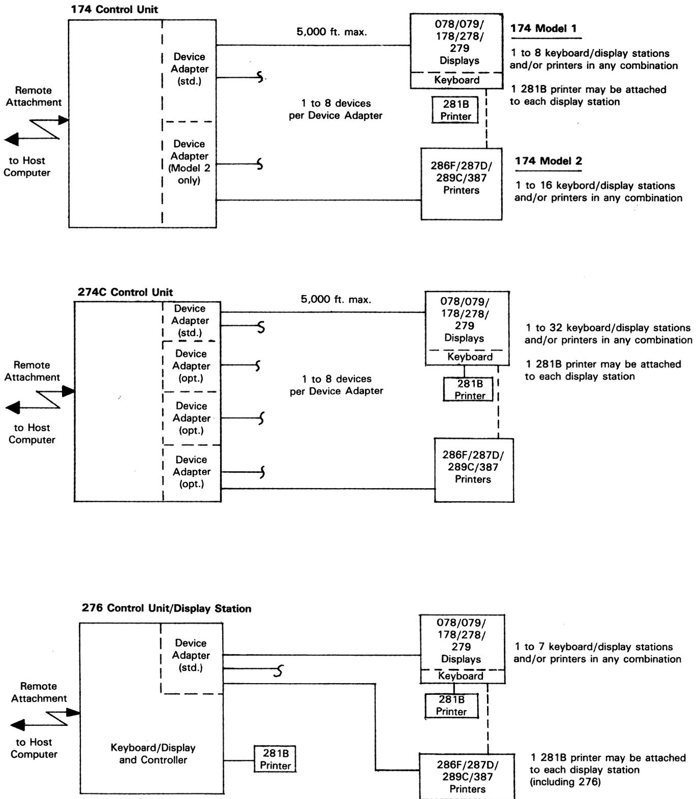
Note: Telex controllers support attachment of IBM displays and/or printers.
