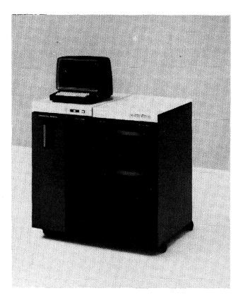
The B 867-1 System and Communications Processor accommodates seven communications lines, and up to 114K bytes of main memory. On the right is a dual cartridge disk drive.
