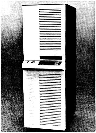
Honeywell's DATANET 6661 network processor is offered as a front-end for Honeywell mainframes in pre-DSA network environments. It supports large and very large systems that run GCOS, GCOS 8, or Multics operating software.
