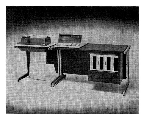
The latest in Datapoint's look-alike family of intelligent terminals and small business systems is the 1150. It is shown here with the company's own "Freedom" matrix printer and two standard and two optional diskette drives. The 1150 is built around Datapoint's most powerful processor, the 5500, but lacks the flexibility of a 5500 system to handle multi-user processing.
