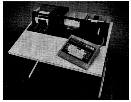
Tab Products' buffered keypunchverifiers use the same keyboard layout as the IBM 129 Card Punch and offer a number of worthwhile additional features. lators. User interest is also developing in utilizing the 501 as a card punch via the bisynchronous communications capability of the unit.
