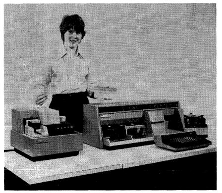
This Decision Data 8010 Interpreting Data Recorder is shown with the optional 96-to-80-Column Card Converter (at left). The 8010's dual input hoppers can be seen at the far right, while the dual output stackers are clearly visible to the left of the keyboard.
