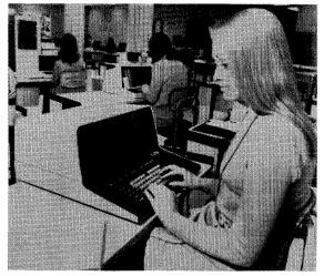
The Key-Edit 50 system can include from 4 to 16 of these CRT keystations, located up to 500 feet from the processor. The Key-Edit 60 system supports a maximum of 24 keystations, some of which can be located up to 6,000 feet from the processor.
