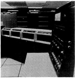
The CDC 33801 Disk Subsystem provides up to 12.8 billion bytes of storage for users of IBM System/370 Model 145 and larger computers.
