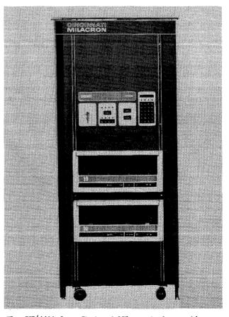
The CIP/4400 from Cincinnati Milacron is shown with a programmer's panel/debug console and two front-loading cartridge disk drives. The CIP/4400 processor can be purchased alone with 32K bytes of main memory for \$16,100, or in a packaged version, the Model 80, with 64K bytes of memory, a CRT, 10-megabyte cartridge disk drive, printer controller, and interface for up to eight CRT's for \$42,800.
