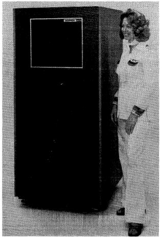
The Ampex ARM-2365 main memory unit allows up to 8 megabytes of memory to be attached to an IBM System/360 Model 65 computer.
