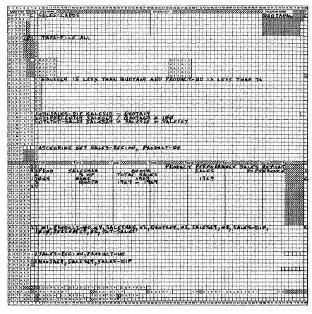
The 16 Score input specifications in this request led to the generation of a COBOL program with 349 source statements. The program, in turn, produced a sales report with seven columns of data, three levels of totals, and an output tape file. A truncated Score input form is shown here to save space. Up to 9 COPY statements, 20 SELECT statements, and 5 COMPUTE statements can be entered on the standard Score form,
