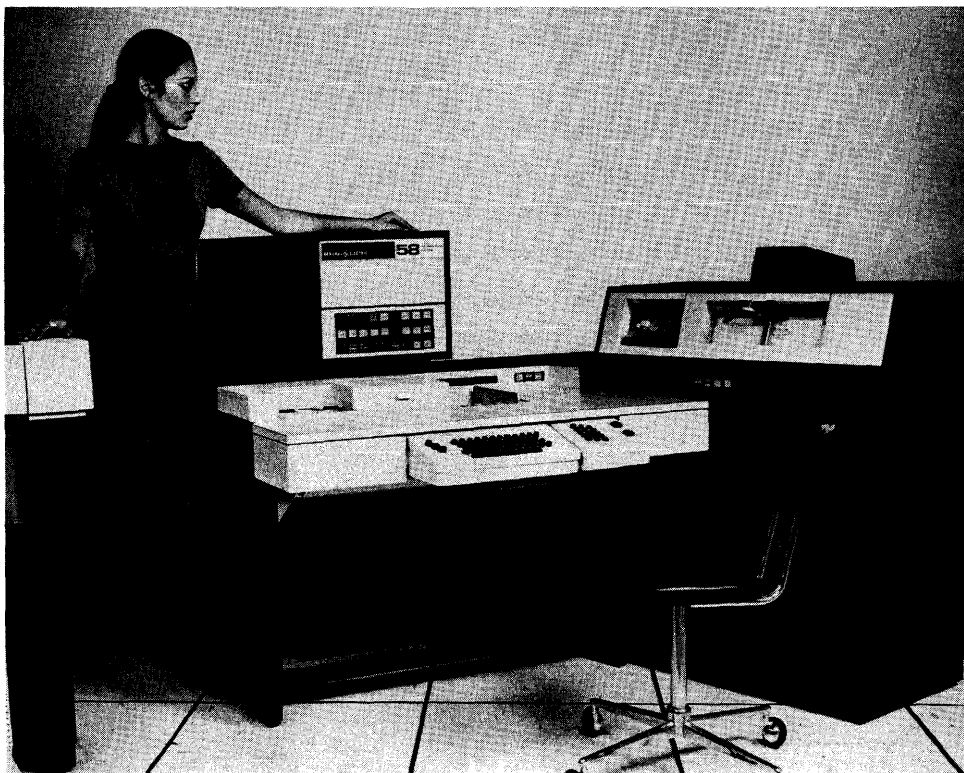
The GE-58 central unit combines processor, alphanumeric and numeric keyboards, card reader, and card punch (at right) in a single compact unit. The associated line printer is at left.
