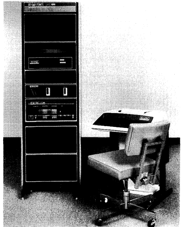
Digital Equipment Corporation's packaged "Standard 8" system consists of a PDP-8/E minicomputer with 8K 12-bit words of core memory, a moving-head disk drive, dual cassette drives, a DECwriter terminal, and software consisting of Digital's OS/8 system and diagnostics. The complete system is priced at $18,000—approximately what the first PDP-8 minicomputer alone sold for when it was introduced in 1965.
