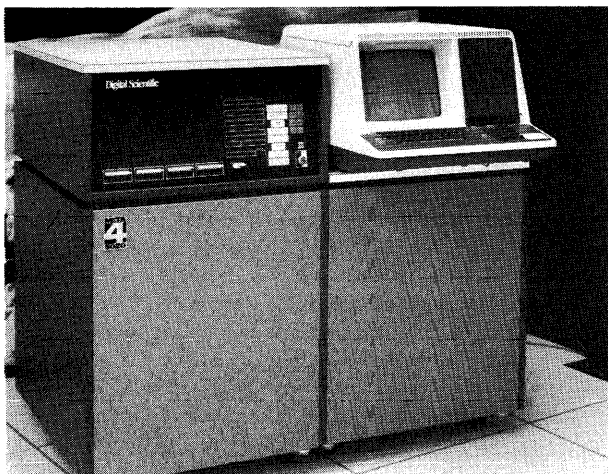
The Meta 4/5020 is one model of the Meta 4 family of micro-programmed computers from Digital Scientific Corporation. This family offers a broad range of capabilities to accommodate a variety of high-throughput time-sharing applications. The 5020 is a midrange member of this family, which extends from a small OEM package to a large-scale system. The purchase price of a basic Meta 4/5020 is $24,500.
