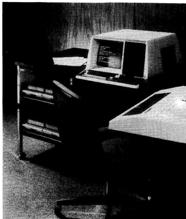
Digital Equipment Corporation's new Datasystem 310 is a complete business data processing system that can be purchased for just $12,000. The basic system consists of an 8K PDP-8/A microcomputer, two diskette drives, CRT display, and keyboard. It can be expanded by adding a printer, a communications interface, more diskette drives, or increased storage capacity. DEC is setting up a distributorship network of software houses that will sell the Datasystem 310 to end users and develop their applications programs.
