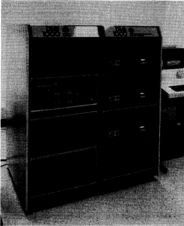
Distribution Management Systems' DMS 1000 is a purchase-only turnkey system built upon the DEC PDP-8/e minicomputer. Featuring COBOL, FORTRAN, BASIC and Assembler languages, the system in a basic configuration can be purchased for $65,500. The operating system supplied with the DMS 1000 allows main memory to be partitioned to handle up to 30 users simultaneously.
