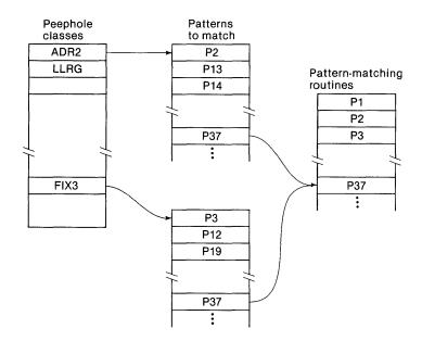
Figure 75. Peephole tables and pattern-maching routines.
