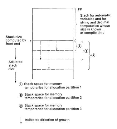
Figure 70. Stack allocation for register temporaries.
