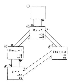
Figure 28. The flow graph of a program's nodes.
