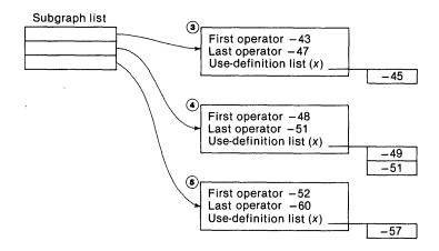
Figure 31. A subgraph for a variable selected for assignment to a register.
