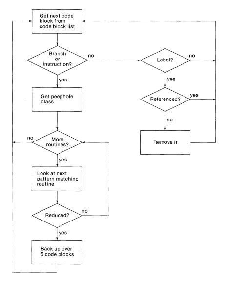
Figure 76. Control flow in the Peephole Optimizer.
