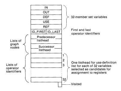
Figure 22. Data in a flow graph node.
