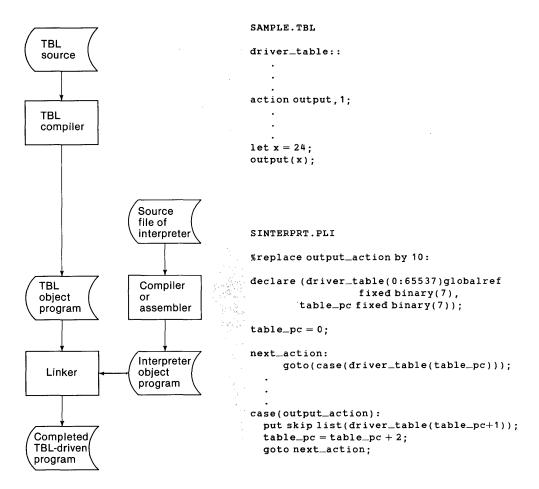
Figure 4. Files required to build a TBL-driven program.
