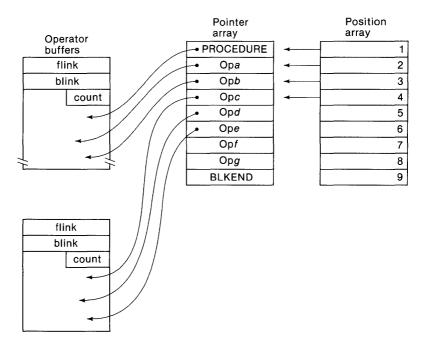
Figure 19. The Optimizer's position and pointer arrays.
