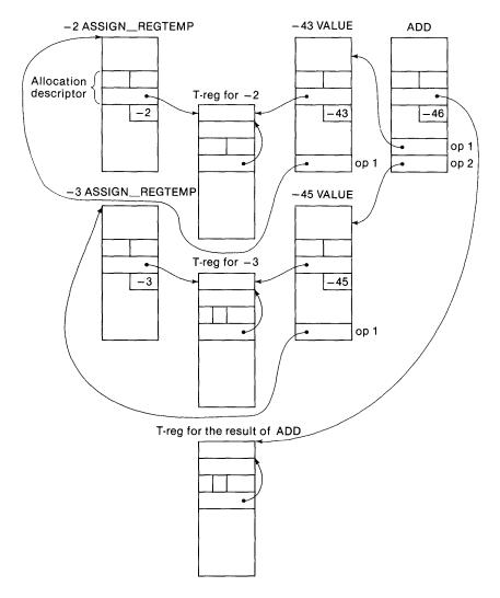
Figure 54. T-reg nodes for ASSIGN\_REGTEMP operators.
