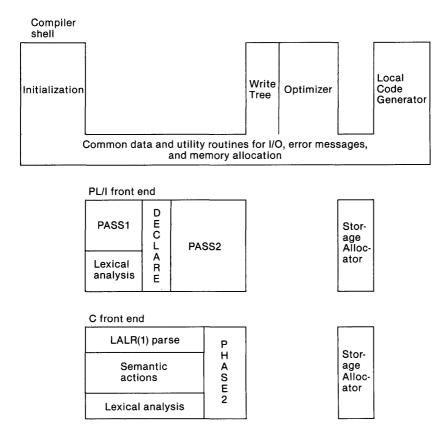
Figure 3. Using the VAX-11 Code Generator for different compilers.
