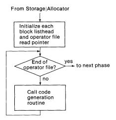
Figure 50. Processing the operator file.
