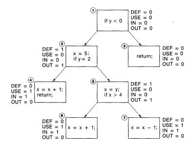
**Figure 30.** Flow graph for a program containing a register temporary.
