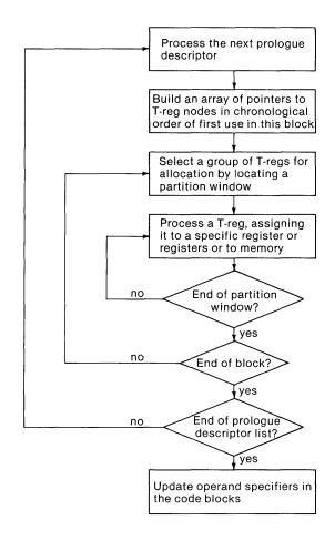
Figure 64. Control flow in the Register Allocator.
