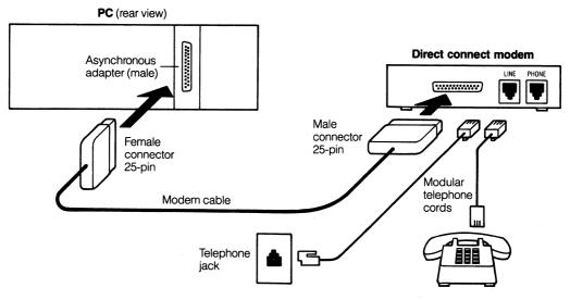
Figure 4-3 A Direct Modem Connection
