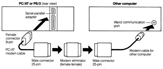
Figure 4-8 (Cont.) Direct Connection, Computer to Computer
