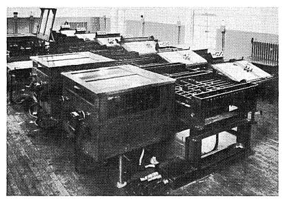
Fig. 2.3 A large differential analyser, designed by D. R. Hartree in 1935. The prototype for this was a small-scale machine built from pieces of children's Meccano construction sets, which actually solved useful equations concerned with atomic theory in 1934.
