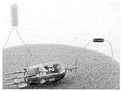
Fig. 4.2 left to right: a germanium semiconductor diode of the 1950s; the thermionic diode of figure 4.1; a silicon semiconductor diode of the 1970s.
