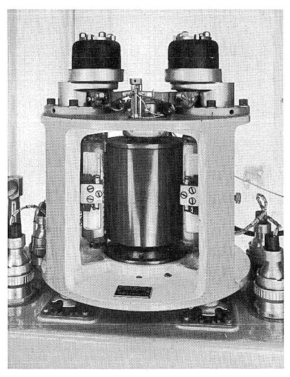
Fig. 4.6 A magnetic drum storage unit from a DEUCE computer (1955). The magnetically coated drum – the dark cylinder in the centre of the container – spins rapidly and information is recorded on its surface by read/write heads at either side. In this particular system the head-structures could be moved vertically to give the effect of many recording tracks.
