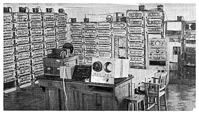
Fig. 7.4 The Manchester University Mark II computer, nicknamed MEG, was 20 times faster than Mark I yet consumed less than half the electrical power. It first worked in May 1954.
