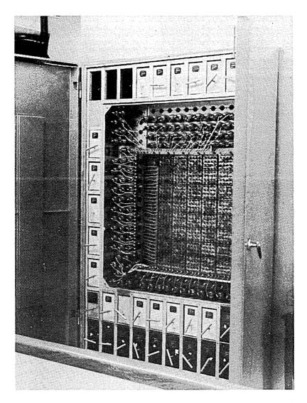
Fig. A1.6 A cabinet of the Cambridge University EDSAC II computer (1957), showing the microprogram control store. The important concept of microprogramming was first expounded by Professor Maurice Wilkes of Cambridge University in 1951.
