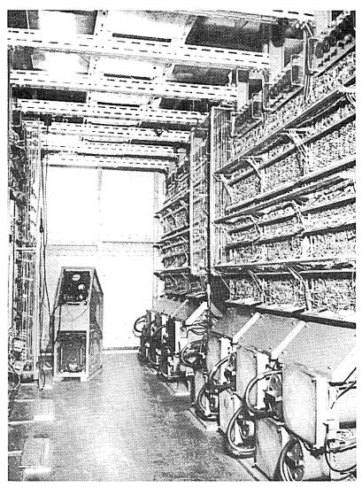
Fig. 10.2 The Telecommunications Research Establishment's TREAC computer, also operational in 1953. This was the first *parallel* electronic computer in the country. The boxes along the lower right side of the machine contain Williams storage tubes. Note the soldering iron conveniently to hand on the left!
