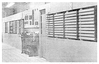
Fig. 12.3 The ICCE relay computer at Imperial College, London University, in about 1952. The electro-mechanical relays are contained behind the horizontal rows of covers. ICCE was the largest of the early British relay computers.
