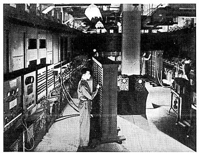
Fig. 16.1 The shape of things to come. A dramatic view of the huge ENIAC electronic calculator, built towards the end of the second world war for ballistics calculations for the US Army. In the foreground an operator sets one of several hundred function switches prior to a computation run.
