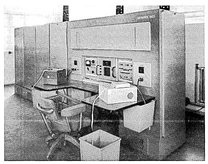
Fig. 9.3 The Metropolitan-Vickers MV950, thought to be the first transistor computer to become commercially available (1956).
