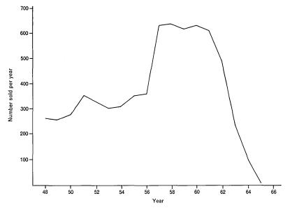
Fig. 14.3 Annual sales of all punched card equipment manufactured by the British Tabulating Machine Company, from 1948–1965. Sales were initially unaffected by the advent of the stored-program computer, especially since most early computers used paper tape for input. In about 1957 computers using cards began to make their presence felt.
