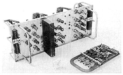
Fig. 14.1 Degrees of modularity: plug-in units from an English Electric DEUCE (left) and a Ferranti PEGASUS computer, both machines designed to facilitate quantity production and allow rapid maintenance.
