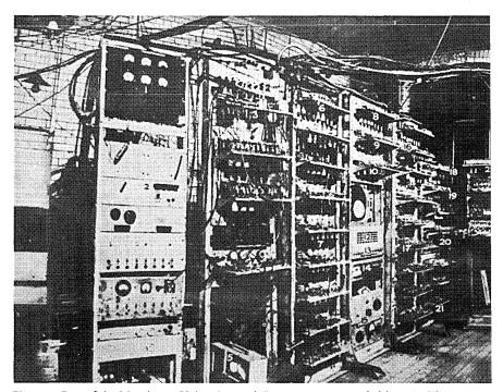
Fig. 7.1 Part of the Manchester University Mark I computer as extended in 1949. The prototype, operational in June 1948, occupied the centre six racks in the photograph and is believed to be the world's first stored-program computer. The Mark I was built out of war-surplus components with an enthusiasm that left little time for tidyness! Incredibly, it worked for long enough at a time for some useful computation to be carried out. It also contained some novel ideas, for example index registers.
