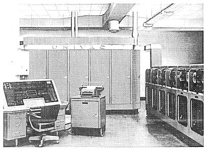
Fig. 16.2 UNIVAC I – the *tour de force* of the Presper Eckert/John Mauchly partnership in computer design. This machine was first installed in June 1951 and was remarkable for its advanced facilities for data handling. To the right of the photograph can be seen some of the magnetic tape decks, of which there could be up to ten.
