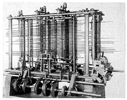
Fig. 1.1 Part of Charles Babbage's Analytical Engine, designed between 1833 and 1837. This remarkable mechanical calculating machine was planned to have a store (or memory) for 1000 numbers, and was to be controlled by punched cards similar to those used in the Jacquard loom. In developing his engine, Babbage conceived the idea of what we would now call a *stored-program* computer.
