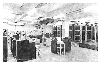
Fig. 13.2 The completed LEO computer, showing the central processor bays in the background to the right of the photograph and the operator's console and input/output equipment in the foreground. LEO was finally switched off in January 1965, at which time it was said to be the oldest operating electronic computer. It had given more than 13 years of continuous service.
