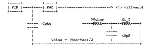
This is designed to approximate a 500hm termination for the purpose of impedance matching for those systems (if any) which drive input clocks across long traces. Furthermore, the high impedance bias driver allows a clock source of arbitrary DC bias to be AC coupled to EV4. The peak-to-peak amplitude of the clock source must be between 0.6V and 3.0V as seen by EV4. Either a "square-wave" or a sinusoidal source may be used. Note that full-rail clocks may be driven by testers.
