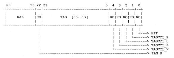
Unused tag bits in the TAG field of this register are always clear, based on the size of the external cache as determined by the BC\_SIZE field of the BIU\_CTL register.
