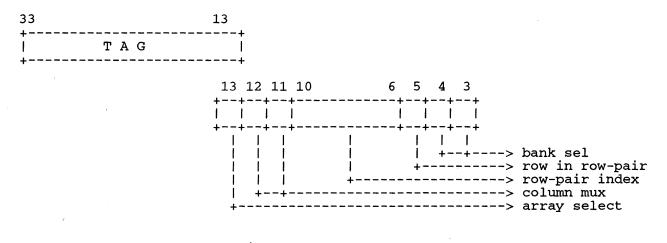
The next figure shows a block diagram of the cache. Each row contains four complete cache blocks; address bits <12:11> control the column mux. The top subarray is selected when address bit <13> is one, otherwise the bottom array is selected. In ICache test modes three and seven, EV45 serially drives the top array's inverted contents onto sRomOe\_l and the bottom array's inverted contents onto sRomOe\_l and the
