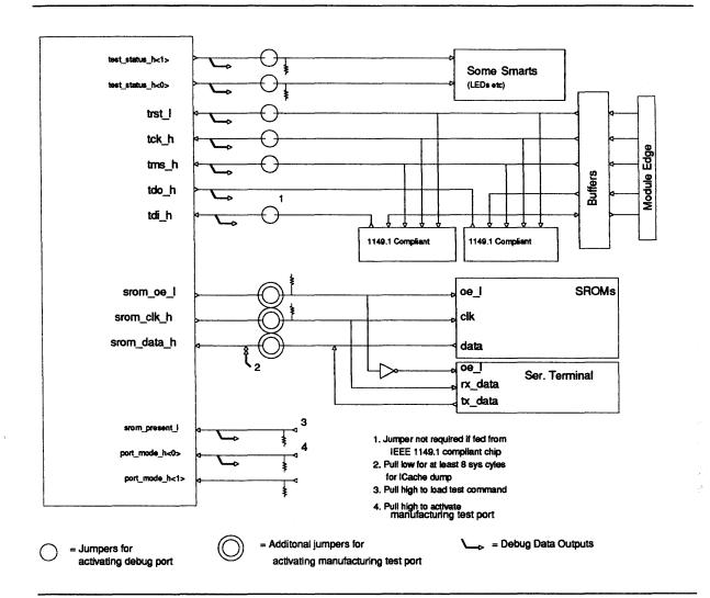
Figure 11-3: Tes Port Connections on Module
