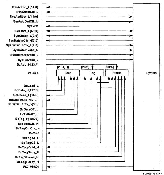
Figure 4-1 21264A System and Bcache Interfaces
