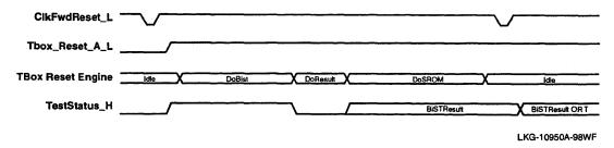
Figure 11-2 TestStat\_H Pin Timing During Built-In Self-Initialization (BiSI)
