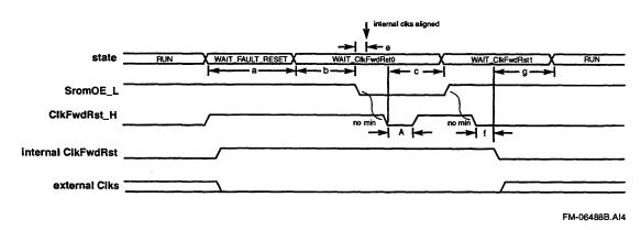
Figure 7-2 Fault Reset Sequence of Operation
