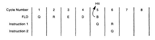
The speculative window for floating-point load instructions is one cycle wide. FQ-issued instructions that are issued within the speculative window of a floating-point load instruction that has missed, are only aborted if they depend on the load being successful.
