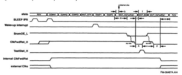
Figure 7-3 Sleep Mode Sequence of Operation
