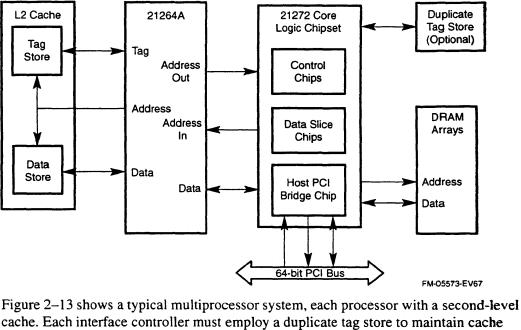
Figure 2-12 Typical Uniprocessor Configuration
