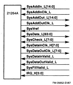
Figure 4-4 System Interface Signals
