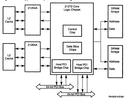
Figure 2-13 Typical Multiprocessor Configuration
