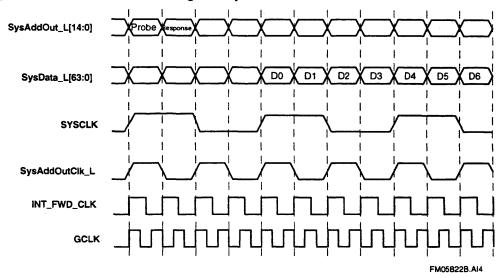
Figure 4-5 Fast Transfer Timing Example
