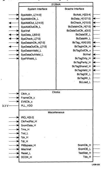
Figure 3-1 21264A Microprocessor Logic Symbol
