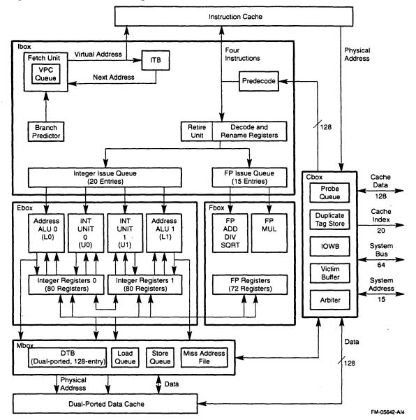
Figure 2-1 21264A Block Diagram
