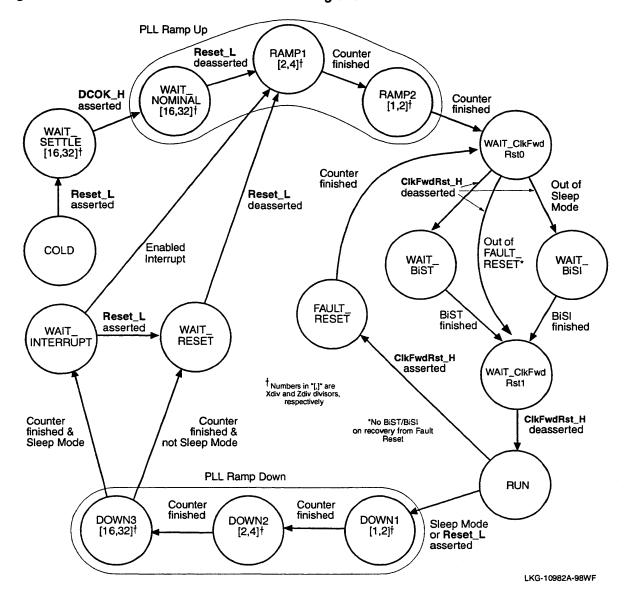
Figure 7-5 21264A Reset State Machine State Diagram
