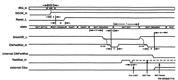
Figure 7–1 Power-Up Timing Sequence
