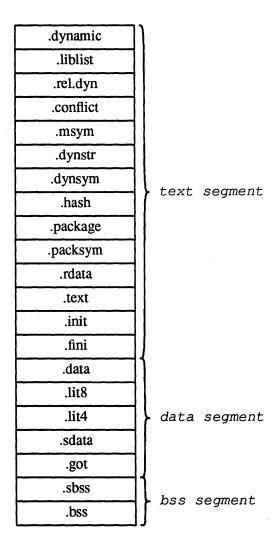
As noted in Figure 9-2, the sections are grouped into the text segment (containing the .text, .init, and .fini sections), the data segment (.rdata, .data, .lit8, .lit4, and .sdata), and the bss segment (.sbss and .bss). A section is described by and referenced through the Section Header; the Optional Header provides the same information for segments.
