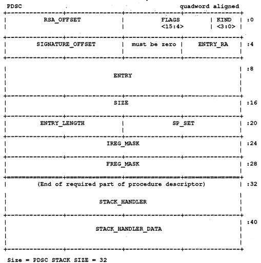
Figure 4–1: Stack Frame Procedure Descriptor Format
