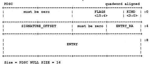
Figure 4-7: Null Frame Procedure Descriptor Format
