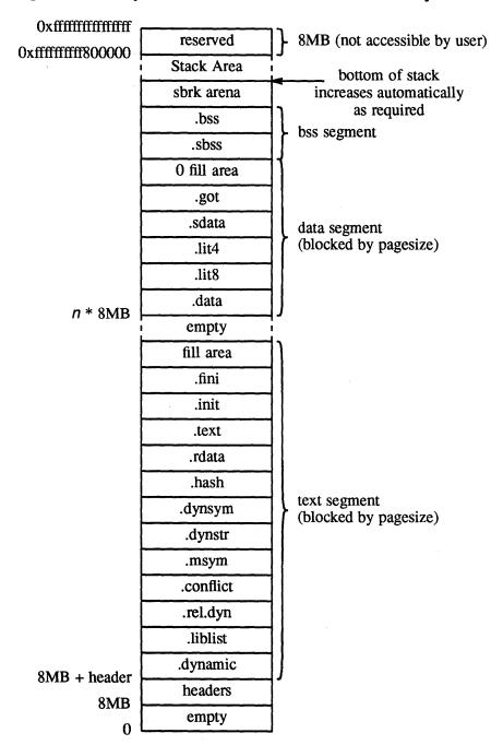
Figure 9-7: Layout of ZMAGIC Files in Virtual Memory
