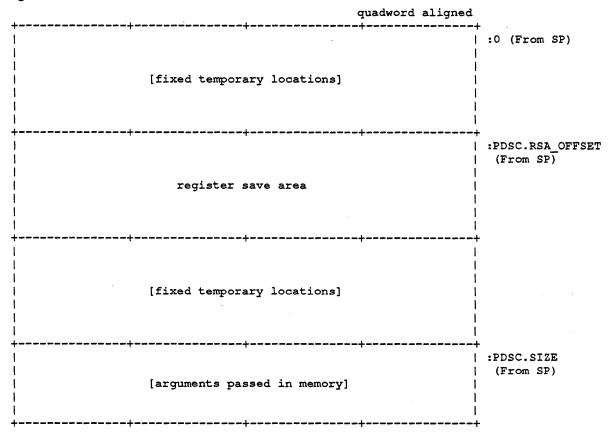
The following figure illustrates the format of the stack frame for procedures with a varying amount of stack which use the FP as the stack base register (i.e. PDSC.FLAGS.BASE\_ REG\_IS\_FP is 1).
