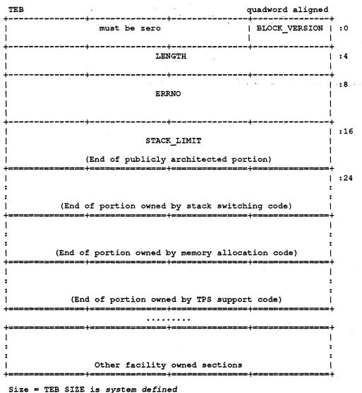
Figure 7–1: Thread Environment Block Format
