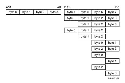
The longword transfers, tribyte transfers, and unaligned word transfers all use the byte lanes in the same way. However, when the low word in a longword is transferred, the data is switched to or from its usual lanes  $\mathbf{D}$ <31:16> to or from  $\mathbf{D}$ <15:0>. Byte transfers in the low word of a longword are swapped in a similar way.
