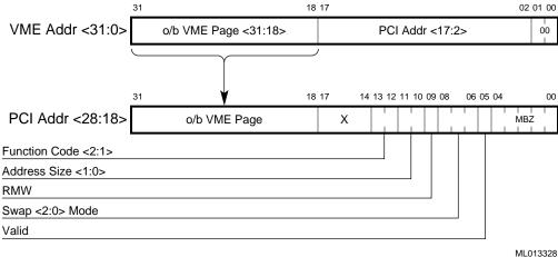
A PCI memory access in either VME WINDOW 1 or VME WINDOW 2 address windows causes a lookup for the corresponding scatter-gather entry. That is, if PCI Address bits <31:29> match the VME\_WINDOW\_1\_BASE register or if PCI Address bits <31:26> match the VME\_WINDOW\_2\_BASE register, a scatter-gather lookup occurs.
