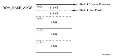
The flash ROM can be rewritten. To protect the flash ROM from unauthorized /accidental updates, a hardware switch must be closed before write operations are enabled. The switch, DIP switch 2 on the Digital Alpha VME 4 assembly, must **always** be open unless flash ROM is going to be updated. The state of the switch is stored in the Flash Switch bit <3> of the module control register.
