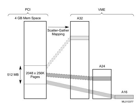
Figure 10-3 Mapping Pages From PCI to VME
