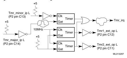
The clock inputs to timer #1 and #2 are a fixed 10 MHz source. The clock input of timer #0 is from a P2 pin (TMR\_MINOR\_IP L) only.
