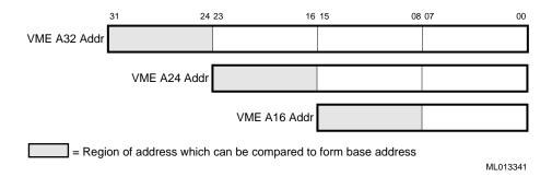
Associated with each of the top three comparison bytes is a bit mask to control the number of bits that are checked during a VMEbus address match. These bits are contained in VIF\_MASK at VME\_IF\_BASE + 0x180. If a bit is set, the address-to-base register bit is not used in the address comparison. At least the top five bits of the A32 address match byte must be used for matching.
