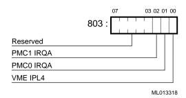
Figure 11-4 Interrupt/Mask Register #3
