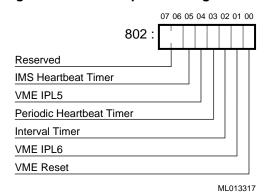
Figure 11-3 Interrupt/Mask Register #2
