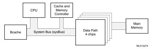
The components of the cache and memory subsystem are distributed between the DECchip 21071-CA and the DECchip 21071-BA. Together, the chips are the interface between the system bus, main memory, and the Bcache (see Figure 6-2).
