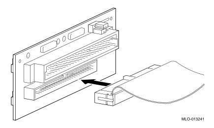
10. Install the primary breakout module (refer to Figure 2-10). Ensure that the breakout module is installed behind the slots occupied by the Digital Alpha VME 4 module (as shown).
