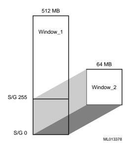
Each page can be mapped to any one of the three VMEbus address spaces: A32, A24, or A16. As shown in Figure 10-3, numerous pages can be mapped to the same VMEbus address to allow access to the same location with different modes. The address modifier code is fully programmable for each page.
