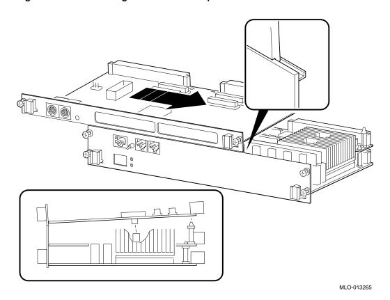
Figure 2-16 Installing the PMC I/O Companion Card
