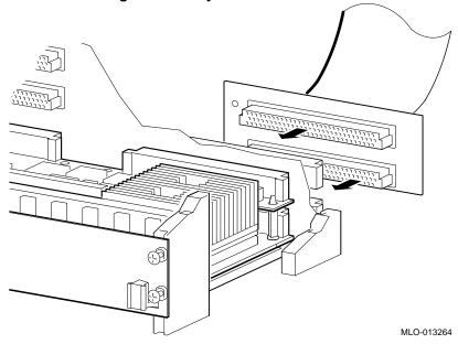
11. A secondary breakout module is included in the hardware kit, which you can connect to the primary breakout module. If you use the secondary breakout module, set the jumpers on that module as shown in Figure 2–11.
