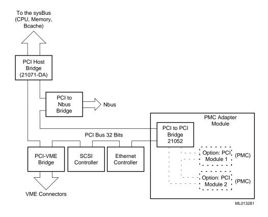
The base address of each PCI device, except the Nbus interface (SIO), is configured by the Digital Alpha VME 4 firmware. Each base address is initialized by writing configuration registers located in PCI configuration space of the system address map.
