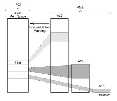
Figure 10–6 Mapping Pages of Memory from VMEbus to PCI Bus
