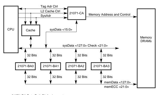
21071-DA Data Path Bit Assignments sysData Lines | memData Lines
