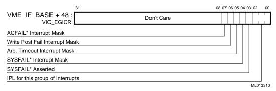
Finally, a local (on-board) interrupt is generated by the VIC64 chip when the VME interface detects a VMEbus IACK cycle to itself. The VIC64 chip can notify the CPU when the VME interface, as a VMEbus interrupter, has its interrupt acknowledged. Once again there is an associated ICR, VIC\_VIICR (see Figure 11–12), to set the IPL and allow the condition to be disabled from generating its local interrupt.
