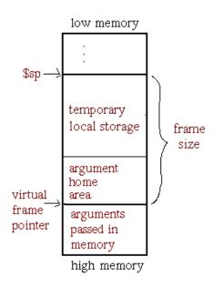
Figure 5–12: Variable-Size Stack Frame
