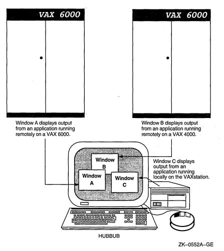
Figure DCLII–1 Running Remote and Local Applications
