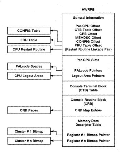
All offset blocks must be at least quadword aligned. The starting address of an offset block is determined by adding the contents of the HWRPB offset field to the starting address of the HWRPB. For example, the starting address of the MEMDSC block is given by:
