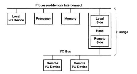
As shown in Figure 8-1, processors and memory are connected by the PMI.
