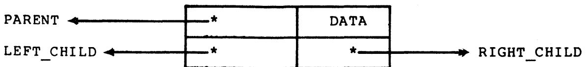
where the pointers for this discussion are offsets into the storage vector rather than an actual address. As such, this configuration can be used to define a binary tree (each parent having at the most two children) as shown below:
