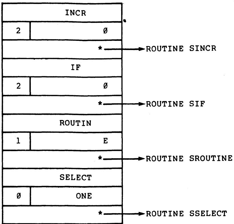
where the names would be in Radix-50. An arrow ( $\longrightarrow$ ) indicates a pointer to the specified data.
