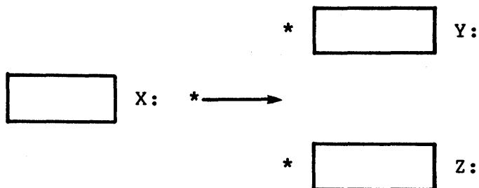
where the condition (depicted by the arrow) acts as a switch to direct either the contents of Y or Z to be transferred to X. The code in most languages would be equivalent to:
