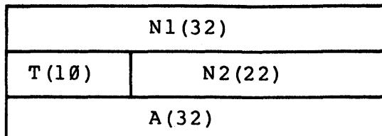
In the above diagram, N1 is the Radix-50 representation of the first six letters in the name; N2 is the Radix-50 representation of the last four letters, T is a type field giving information about the name; and A is the address of the routine which processes that name. To keep this example simple, only four names of this table will be initialized. The following macro initializes the block:
