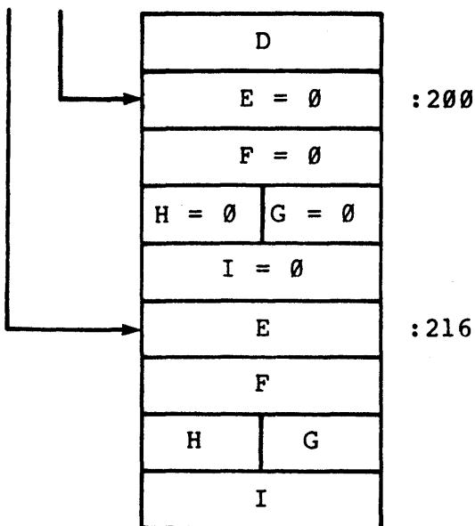
where A through D represent the data fields for the initial fixed blocks, and E through I represent the data fields for the supplementary data block. Note that the first fullword of each initial block is a pointer to the additional data block and that those with no additional data point for compatibility to a common block which is preset to zero.
