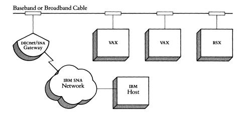
Each DECnet/SNA Gateway can handle up to two lines to remote SNA networks. In network applications with extremely heavy traffic between the DECnet and SNA environments, more than one DECnet/SNA Gateway may be necessary.
