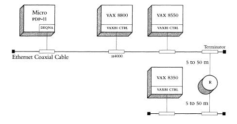
If it is necessary to expand the network to another building up to 1,000 meters (3,280 feet) away, a remote repeater is necessary as shown in Figure 2.43. Notice that the remote link uses a fiber optic cable.
