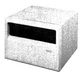
The DFM Series of Intelligent Communication Processors (ICP) are free standing units that utilize statistical time division multiplexing techniques for concentrating four to sixteen EIA RS232C data channels over a single high speed communication link. These data channels interface to terminals, personal computers, workstations, modems, and computer ports.
