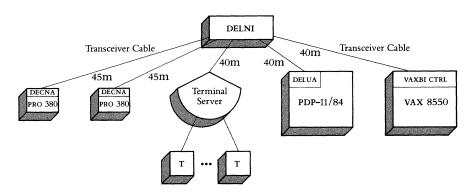
The DELNI hierarchical standalone configuration, illustrated in Figure 2.59, supports a combination of DELNIs and devices using standard Ethernet transceiver cables up to 50 meters (164 feet) away for other DELNI and between 40 and 45 meters (131.2 and 147.6 feet) depending on the communications controller. The DELNI hierarchical standalone configuration is not connected to the Ethernet coaxial cable.
