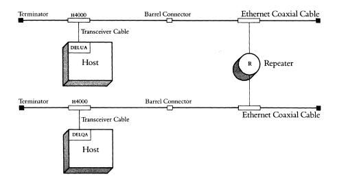
Figure 2.2 Basic Broadband Ethernet Cabling Layout
