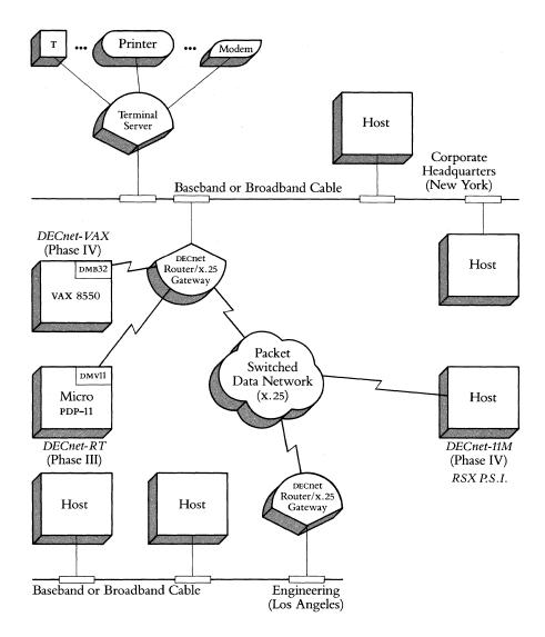
Two lines on each DECnet Router/x.25 Gateway are reserved for configuration as x.25 lines. These lines are the first two in each server box.
