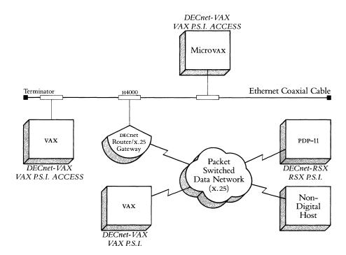
Figure 3.12 X.25/X.29 Terminal Access Configuration
