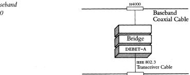
Figure 2.27 Baseband-to-baseband LAN Bridge 100 Configuration
