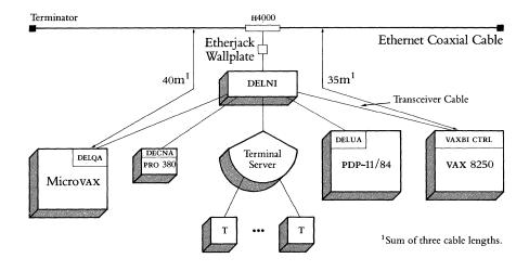
Figure 2.62 DELNI Connected Configuration (Broadband)
