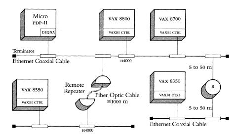
Standard Ethernet (Baseband) Distance Guidelines Standard Ethernet is a branching non-rooted tree topology with a maximum node separation (the distance between the two furthest systems on the network) of 2.8 kilometers (1.74 miles). Up to 1,023 transceivers can be connected to the Ethernet coaxial cable, allowing connection of thousands of devices.
