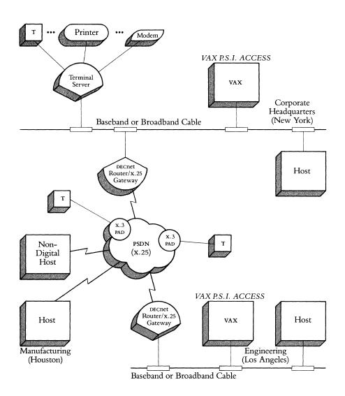
The VAX P.S.I. Access Software provides the following capabilities to VAX hosts on an Ethernet LAN:
