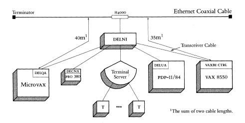
Figure 2.22 DELNI Hierarchial Connected Configuration
