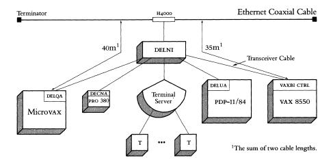
In configurations with an Etherjack (baseband only), the lengths to be considered are from the H4000 to the Etherjack, Etherjack to DELNI, and DELNI to the host system or communications server.
