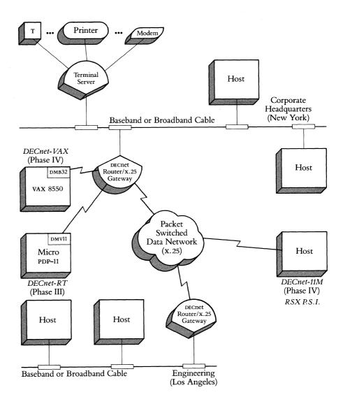
At least one VAX/VMS host system on the Ethernet LAN must have a copy of the basic DECnet Router/x.25 Gateway software. This host system downline loads the software into the DECnet Router/x.25 Gateway. Then the DECnet Router/x.25 Gateway is started up and DECnet-to-DECnet communications are available to all other host systems on the Ethernet LAN.
