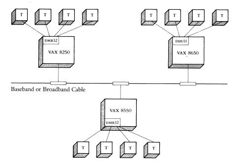
Terminal Servers allow a more flexible connection scheme than direct connection. A group of terminals connect to a terminal server, which then connects directly to the Ethernet LAN, allowing the terminals to access any host on the LAN. Printers and modems can also connect to a terminal server, allowing them to be shared by all host systems on the LAN. Terminal servers can be placed close to the users' workplace, thereby reducing the length of wire extending from each terminal.
