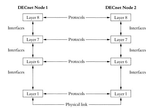
A major advantage of the DNA structure is that the layers are independent of each other. Each layer can be changed without significantly affecting other layers. The unique adaptive quality of DECnet software is the result of DNA's layered structure. DECnet software is especially important because it allows Digital to adapt DECnet to include new communications technologies, such as Ethernet, without affecting the user's applications.
