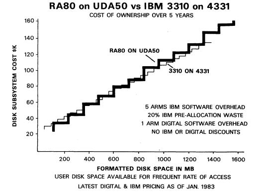
The RA80 is competitive when compared to IBM's low-end fixed disk.
