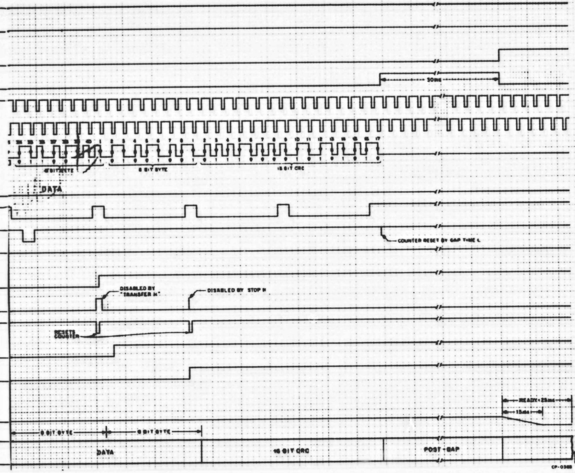
Figure 4-8 Write Timing
