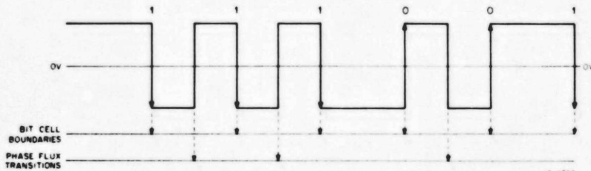
Figure 4-7 Typical Phase Encoded Waveform
