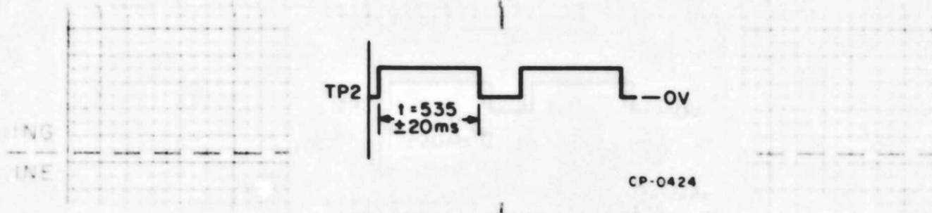
Figure 5-9 Write File Gap Waveform
