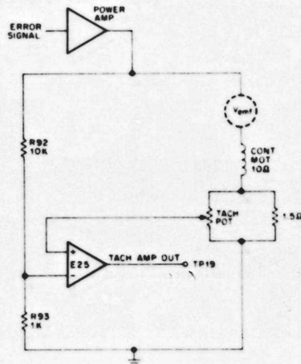
Figure 4-12 Tachometer Circuit
