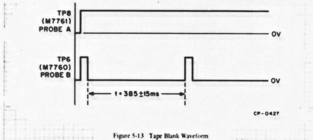
Figure 5-13 Tape Blank Waveform
