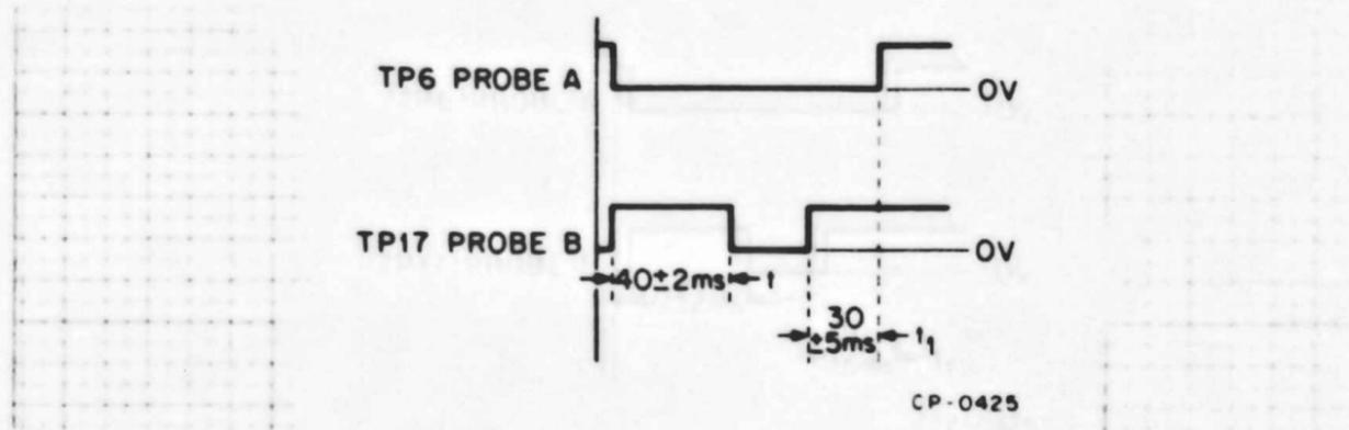
Figure 5-10 Gap Time Waveform
