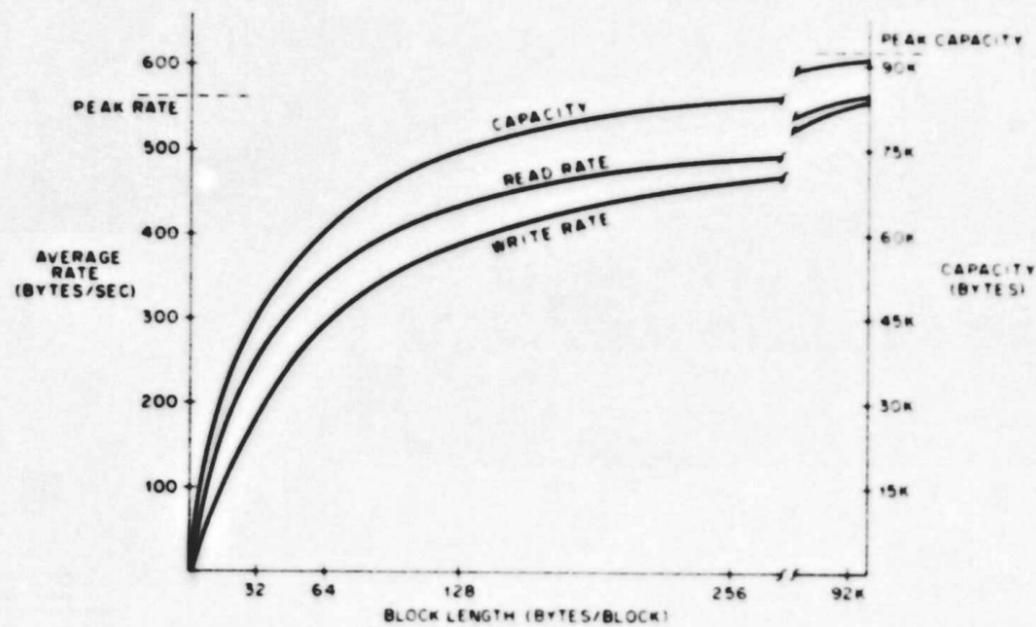
Figure 1-1 Capacity and Data Rate vs Block Length
