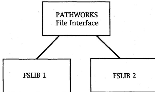
Figure 1. File system top level structure
