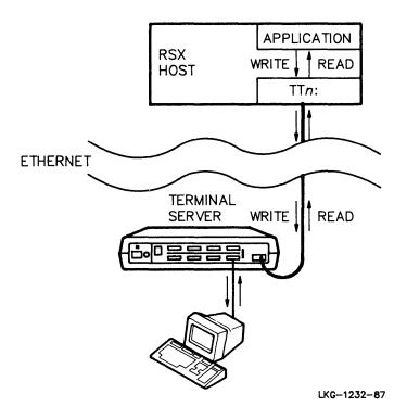
Figure 6–2 gives a more detailed picture of the components that make it possible for applications to communicate with remote LAT devices.
