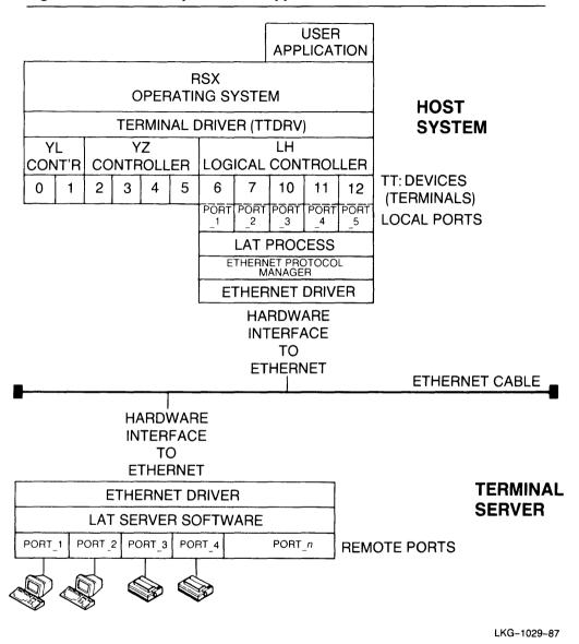
The terminal server is a piece of hardware that has a physical connection to the Ethernet. It also has connections to devices such as user terminals, printers, and so on. A device attached to the terminal server is the target of your application.
