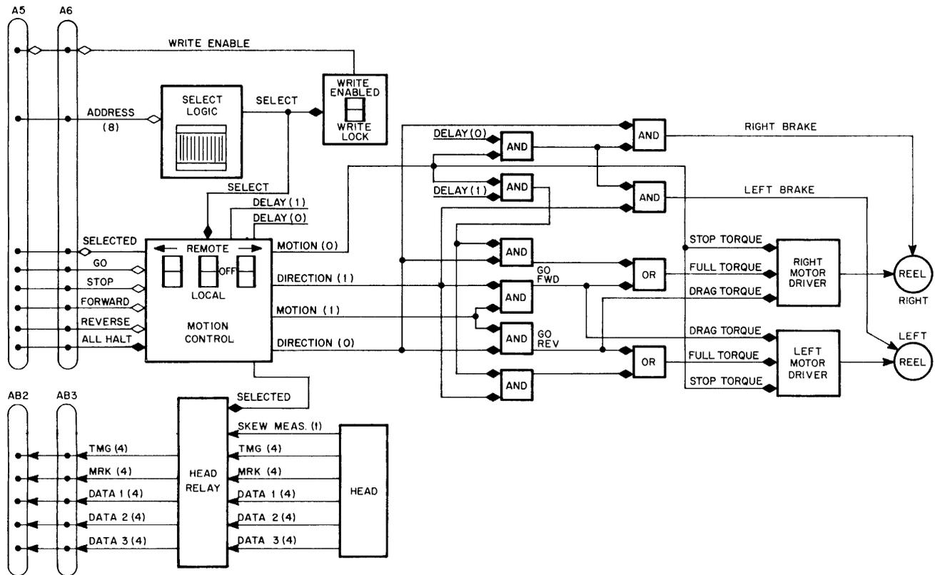
NOTE: An arrow signifies a nonstandard DEC signal, such as motor voltage, head playback, brake voltage, etc.
