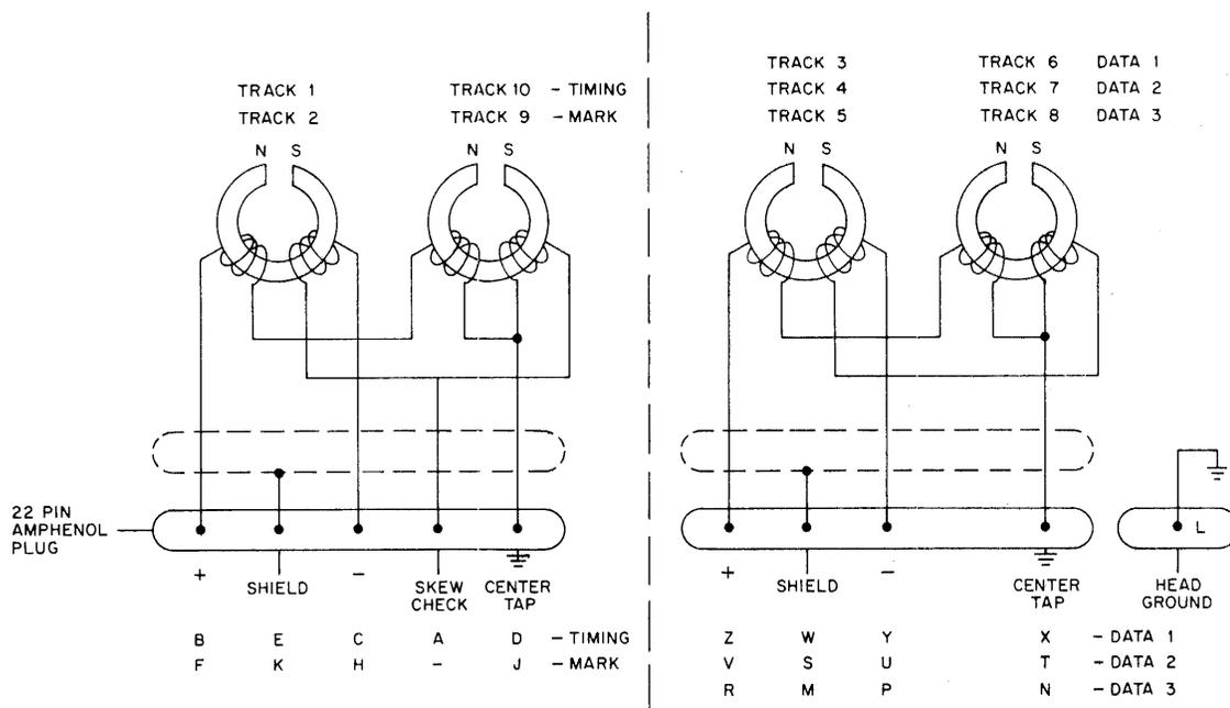
Figure 2-2 Head Connections
