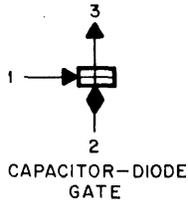
CAPACITOR-DIOLE GATE, POSITIVE OR NEGATIVE INDICATED BY POLARITY OF THE INPUTS.
