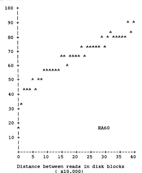
There are several things which are worth noting. The first is the relative performance of the drives. Performance in this test is defined as the speed the drive can read one block and then a second n blocks away. From the curves, it is obvious that the RA81 has better performance than the RA80, which is slightly better than the RA60, which is somewhat better than the RM02. If you calculate the average access over the range of blocks tested, you get the following numbers:
