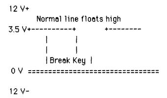
I soon discovered these unexpected BREAK events occurred whenever the SEL lost a "?" character in the VAX KERMIT packets. This was unexpected since typing in "?" worked fine. Something about "?" in a 9600 baud block made the SEL detect a break.
