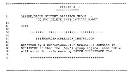
Figure 3: Input file for creating the OPERATORn group logical name table (see Fig. 2).
