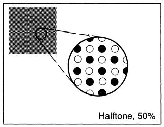
Figure 1. Grays are simulated by half-toning for bi-tonal printers.
